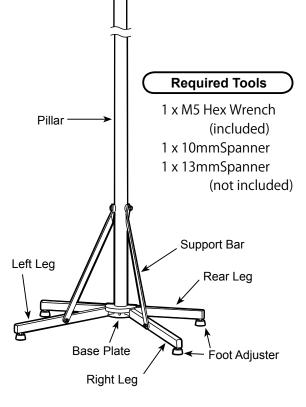
Assemble Right and Left Legs to Base Plate with the supplied M6x35 bolt, Washer, Collar
