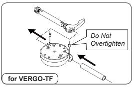
For mounting a 12mm thru axle type
